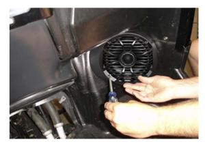
After attaching the speaker wires to the speaker install the speaker into the Wet Sounds Works kick panel after the 4 screws are secured secure the grill over the speaker
