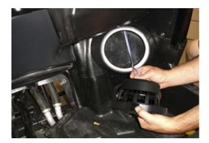
After securing the allen bolts with the  $7\!/16$  nuts run your speaker wire into the kick panel
