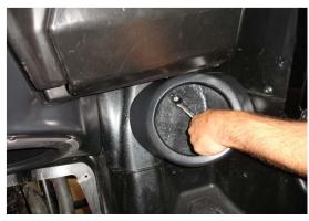
Once all the holes are drilles, mount the kick panel in the RZR, we recommend putting the nut on the inside of the kick panel
