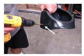
Drill a hole in the top of each kick panel, this is where the speaker wire will run out of. Sealing this hole will give you more sound from the speaker
