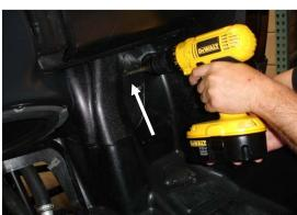
After marking the holes, drill the mounting holes using a 1/4" drill bit
